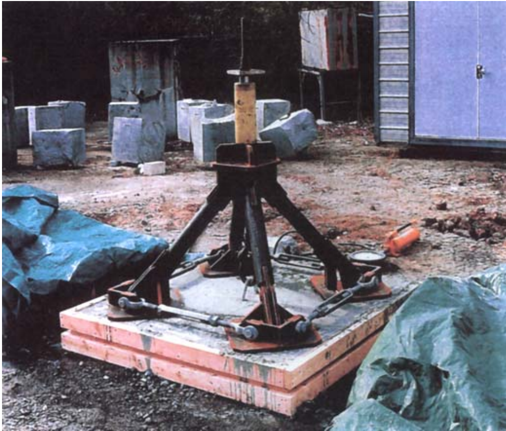
Photo 4. Load frame, ram, and jack
